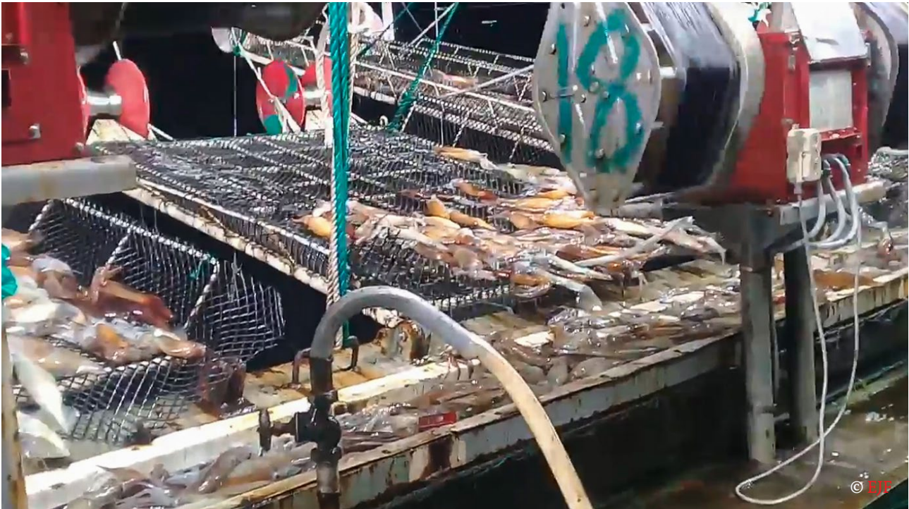
Image showing how squid are brought on board after being caught by automatic squid jigging machines – Chinese-flagged vessel operating in the Southwest Atlantic.
