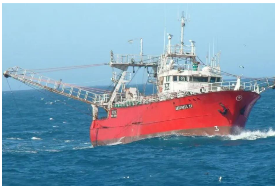
Fig. 43. Shrimp vessel - Arbumasa XV. Bottom trawl net with outriggers (Source: ARBUMASA S.A.)
